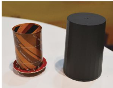
THE HELICAL antenna in both housed (right) and unmounted form.
